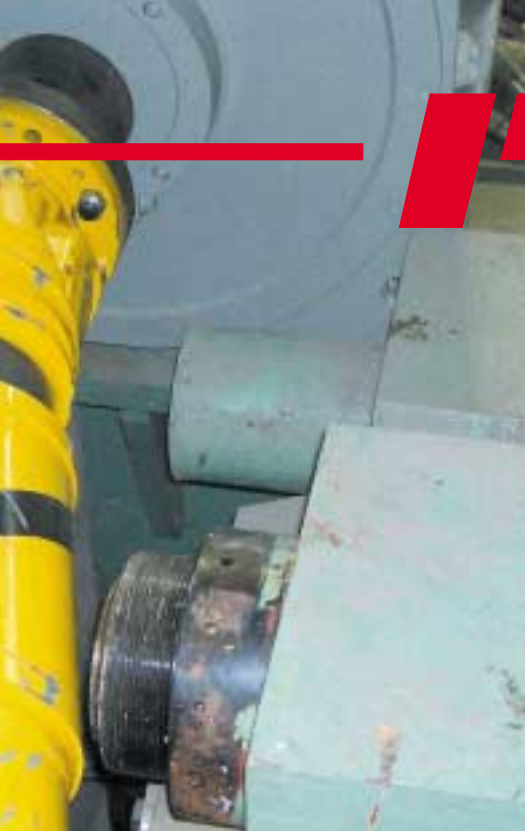
ITH-Tension Nut TN 140 Pre-tensioning of expansion bolts M 140 x 6 in a confined space on a rolling-mill stand.
