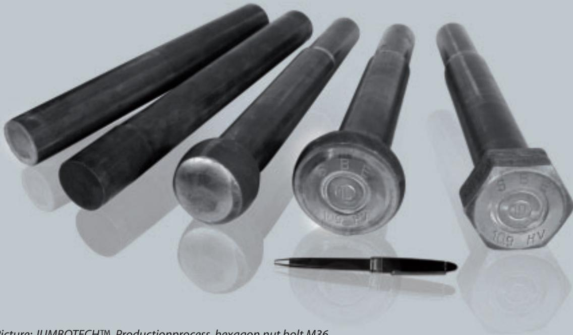
Picture: JUMBOTECH™ Productionprocess, hexagon nut bolt M36
